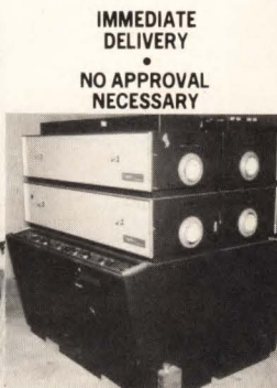
VIEW OF DIFFUSION TUBU- LAR MUFFEL FURNACES
